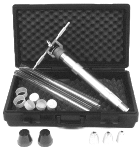
Hand corer with two lexan nose pieces; two liner tubes with caps; three eggshell™ core catchers.
